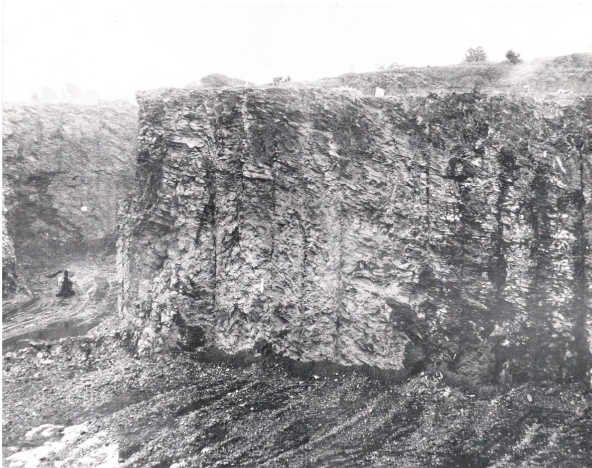
BLASTING SEQUENCE FOR BOTTOM PRIMING QUARRY FACE BEFORE INITIATION COURTESY OF ATLAS POWDER COMPANY
